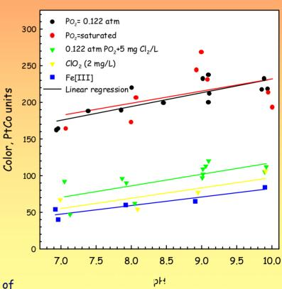
The effect of oxidant type on the color of iron particles collected from filter backwash.
