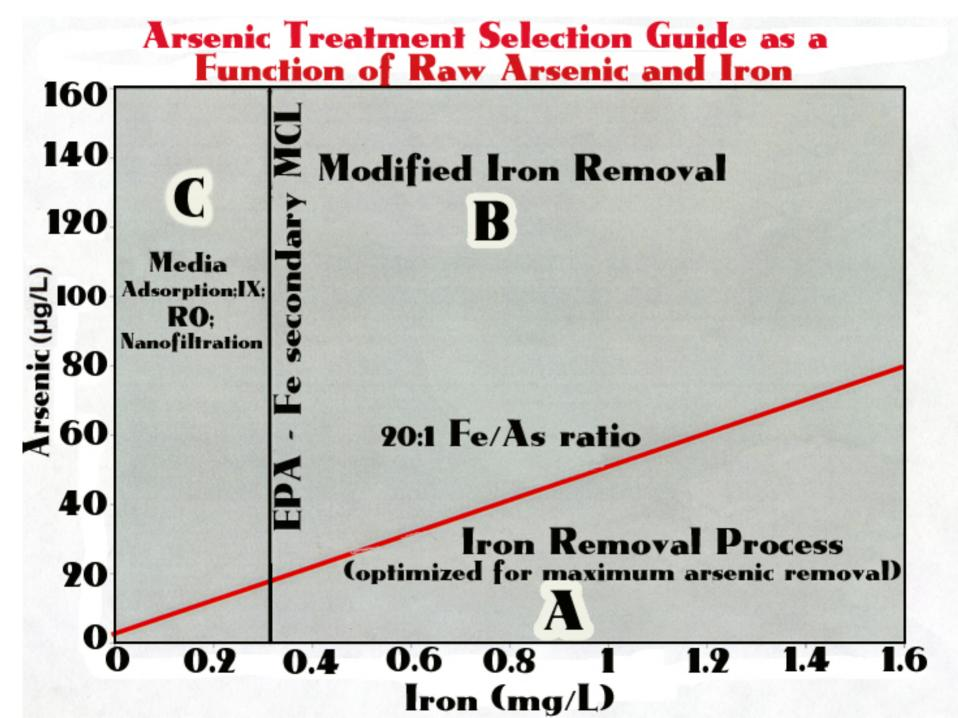
Arsenic Treatment Selection Guide as a Function of Raw Arsenic and Iron 160 140 **Modified Iron Removal** 120 Media Arsenic (µg/L)
